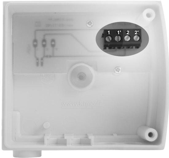
**Cable connection on terminal block**
